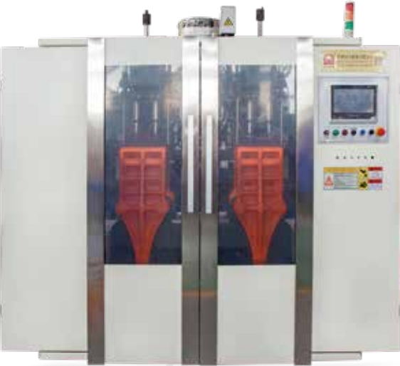
HTSII-2L FULLY AUTOMATIC EXTRUSION BLOW MOLDING MACHINE
