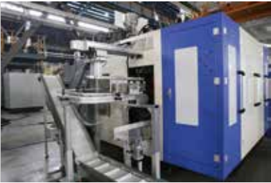
HS-Waste Material Recycling System
