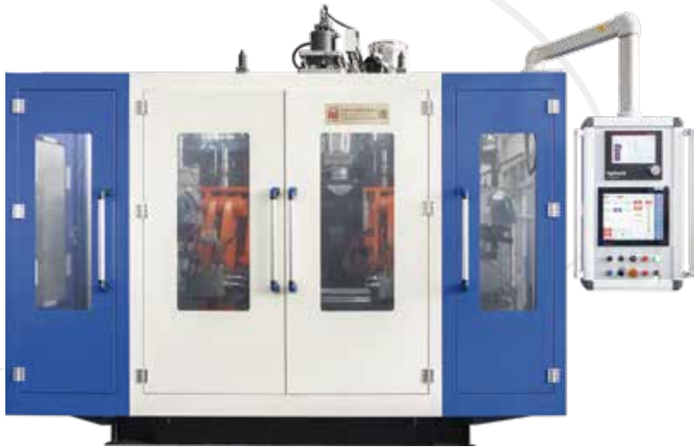
HSII-12L FULLY AUTOMATIC EXTRUSION BLOW MOLDING MACHINE
