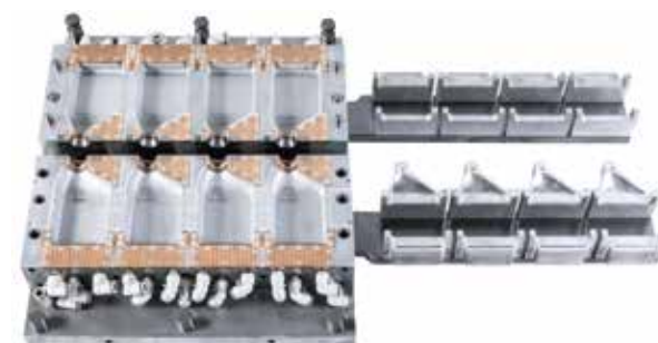
1 L four-cavity deflashing mold
